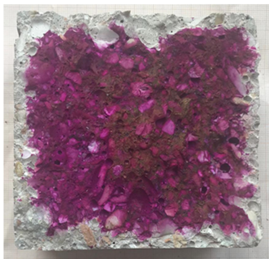
Figure 7. Carbonated specimen after phenolphthalein test.
