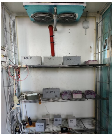
Figure 6. Accelerated carbonation test setup.
